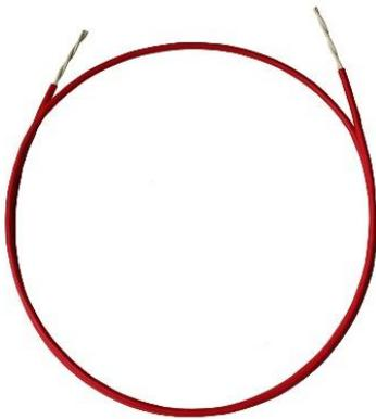
The Context Plus FirePlus-LHD range of digital linear heat detection cables and accessories are designed to monitor and trigger a response when a specific temperature is reached. If the temperature surrounding the cable reaches the activation temperature, the two cores quickly come into contact and trigger an alarm.
