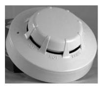
The Context Plus Addressable Optical Smoke Detector. Within the case is a printed circuit board which, on one side, has the light proof labyrinth chamber with integral gauze surrounding the optical measuring system and, on the other, the address
